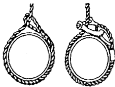
Bad - Because of cutting action of eye splices on running line.
