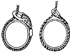
Good - No cutting action on running lines
